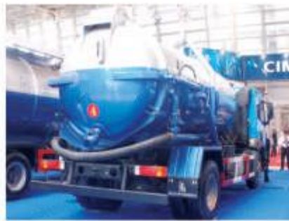
Waste Suction Truck
