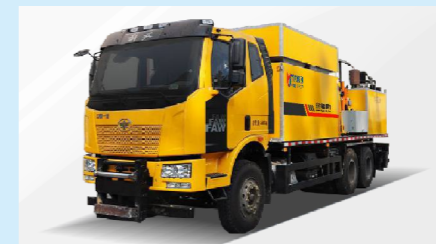
HOT RECYCLED ASPHALT PAVEMENT MAINTENANCE TRUCK
