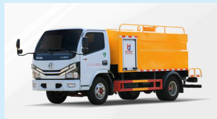
SEWAGE JETTING TRUCK
