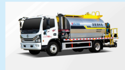
ASPHALT SPREADING TRUCK
