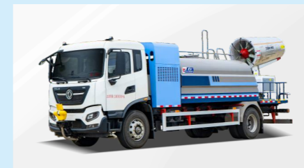
DUST SUPPRESSION TRUCK
