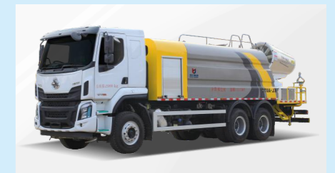
DUST SUPPRESSION TRUCK
