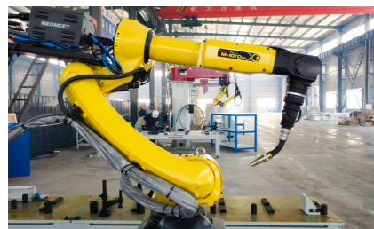
Automatic welding robot
