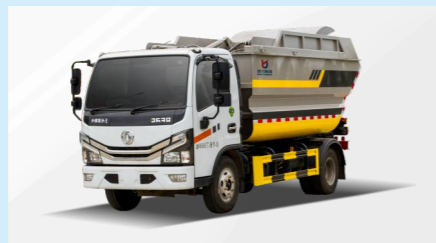
DUMPER PLACER GARBAGE TRUCK
