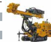
Multifunctional Anchor Drilling Rig
