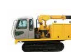
Mobile Welding Station
