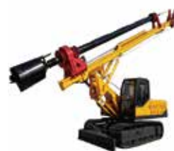
Rotary Drilling Rig
